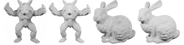
Fig. 10. Reconstruction results on the Stanford raw range scans. Disconnected redundant components in reconstructed mesh caused by outliers are removed manually for better visualization.
